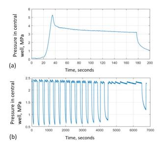
**Fig. 8.** Pressure change in the central well: (a) the formation of a hydraulic fracture during injection with a constant flow rate; (b) cyclic injection with controlled pressure (lower).
