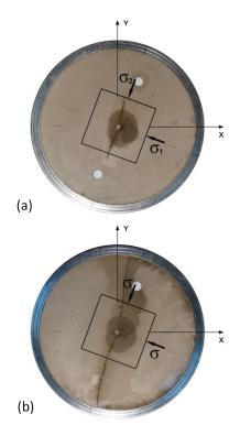
**Fig. 9.** Photo of the sample: (a) hydraulic fracture after injection at a constant flow rate; (b) fracture after injection with a cyclic change in injection pressure.
