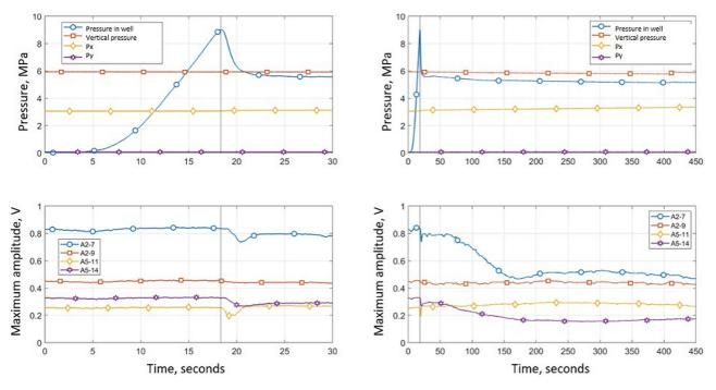
**Fig. 7.** Initial section (on the left) and complete records (on the right) of the dependences of pressure in the central well and loading pressure on time (upper graphs) and the amplitude of ultrasonic pulses for different receivers (lower graphs).
