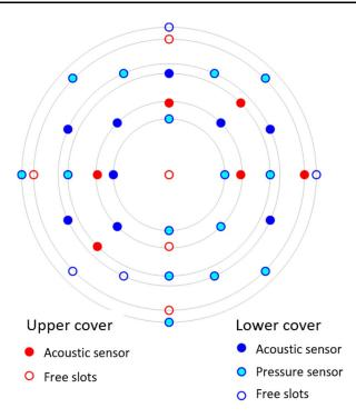
Fig. 3. Layout of pressure sensors and acoustic emission sensors in a top view of the setup.
