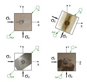
Fig. 4. Orientation of fractures in experiments to determine the influence of pore pressure on the trajectory of fracture propagation. In - an injection well, Out - a production well.
