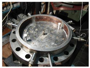
**Fig. 2.** Photos of the hydraulic fracturing simulation setup. On the inside surface of the side ring, chambers for creating horizontal stresses are visible; in the center there is a model well for hydraulic fracturing; on the sides there are auxiliary wells for creating a pore pressure gradient.
