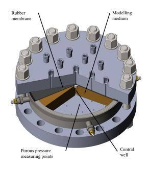
Fig. 1. Diagram of the hydraulic fracturing simulation setup.
